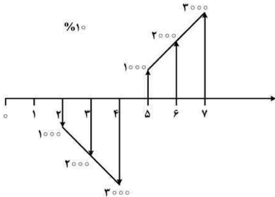
$$\begin{aligned} \left( \frac{P}{F}, 10\%, 2 \right) &= 0.82 \\ \left( \frac{P}{F}, 10\%, 3 \right) &= 0.75 \\ \left( \frac{P}{G}, 10\%, 3 \right) &= 2.33 \\ \left( \frac{P}{G}, 10\%, 4 \right) &= 4.38 \\ \left( \frac{P}{G} = 10\%, 7 \right) &= 12.763 \end{aligned}$$
