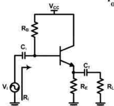
$$R_i = R_B \parallel r_\pi \text{ (1)}$$
