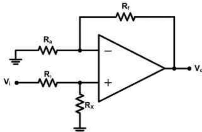
$$A_V = \frac{1 + (R_f / R_a)}{1 + (R_f / R_x)} \quad (1)$$
