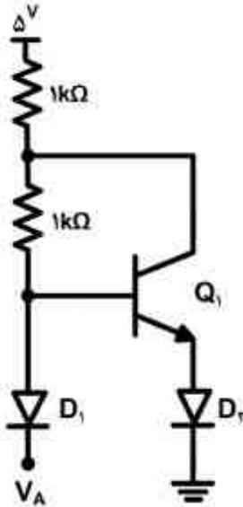
$$\beta = 40, V_{BE} = 0.7 \text{ V}$$
