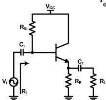
$$R_i = R_B \parallel r_\pi \text{ (1)}$$
