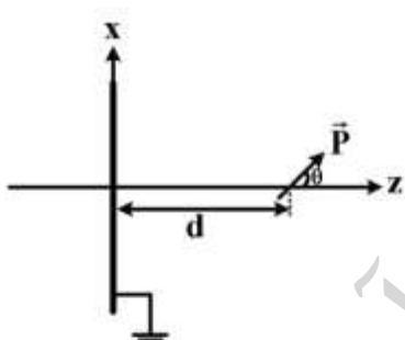
$$\frac{P}{4\pi\epsilon_0} \left\{ \frac{x \sin \theta + (z-d) \cos \theta}{[x^2 + y^2 + (z-d)^2]^{1/2}} + \frac{-x \sin \theta + (z+d) \cos \theta}{[x^2 + y^2 + (z+d)^2]^{1/2}} \right\} \quad (1)$$
