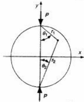
$$\sigma_x = -\frac{2P}{\pi} \left[ \frac{(R-y)x^2}{r_1^4} + \frac{(R+y)x^2}{r_2^4} - \frac{1}{D} \right]$$
