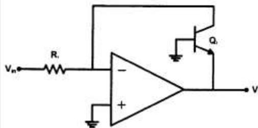
$$V_{out} = -\frac{V_{in}}{R_1} \quad (1)$$
