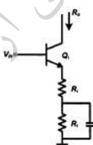
$$R_{out} = r_o + (gm r_o + 1)(R_\gamma || r_\pi) \quad (1)$$
