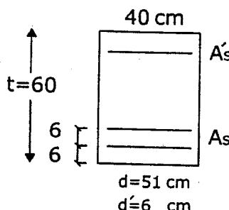
$$f_y = 4000 \text{ kg/cm}^2 \quad f_{cc} = 200 \text{ kg/cm}^2$$
