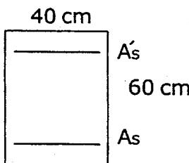
$$f_y = 4000 \text{ kg/cm}^2 \quad f_{cc} = 200 \text{ kg/cm}^2$$
