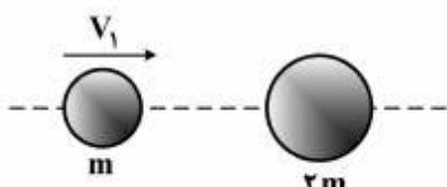
$$v'_1 = \frac{2}{3} v_1, v'_2 = \frac{1}{3} v_1 \quad (1)$$
