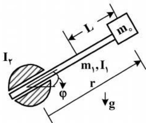
$$\frac{1}{2}I_r\dot{\phi}^2 + \frac{1}{2}I_1\dot{\phi}^2 + \frac{1}{2}m_0[r^2\dot{\phi}^2 + \dot{r}^2] + m_0g(r-L)\sin\phi \quad (1)$$
