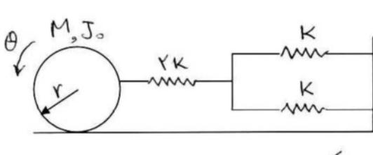
$$\omega_n = \sqrt{\frac{3k}{M}} \quad (2) \quad \omega_n = \sqrt{\frac{k}{3M}} \quad (1)$$
